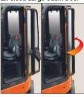
The door opens in two steps and has increased width of 610 mm, allowing
