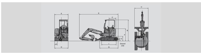
The illustration shows the ZAXIS30U-2 canopy version equipped with 1.17 m arm and 300 mm rubber shoes.
