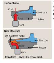
The Hitachi-developed rubber crawlers are highly durable, featuring a steelcored structure that protects shoe edges from being damaged even when riding on curbs.
