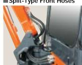
Split-type front hoses are jointed at the machine cover ports and the back of the boom for easy replacement.
