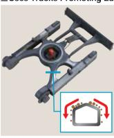
The X-beam track frame is rounded for smooth mud removal. One-sided slope on the side track frame promotes mud sliding-off, minimizing mud packing problem. This shortens machine washing time and reduces disposal costs,
