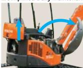
The engine cover can slide up and down for quick servicing even in confined space. No more swing-open cover that obstructs maintenance and servicing jobs. The right side cover swings open for a quick battery check.
