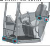
The cabin rests on 4 shock-absorbing rubber mounts to ensure comfortable
