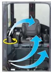
Compact yet ample-capacity air conditioner is provided standard. The full-360° rotatable air outlet also serves as a defroster, maintaining operator comfort all the year round.
