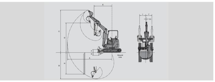
The illustration shows the ZAXIS30U<sub>2</sub> canopy version equipped with 0.09 m³ bucket, 1.52 m arm and 300 mm rubber shoes.
