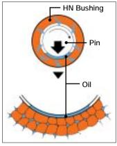
The HN bushing, another example of innovative technology developed by Hitachi, features long life and high durability. High-viscosity oil is vacuum impregnated in sintered high-hardness metal. During operation oil oozes come from the pores of the bushing into the clearance between pin and bushing for self-lubrication.
