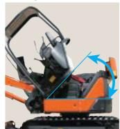
The cabin floor can be tilted up for easy, quick servicing even in the case of an emergency. The floor can be tilted up to 50° to allow the operator to work under the cabin floor. It also gives direct access to the swing mechanism and starter motor behind the engine located under the cabin floor. This design reduces inspection and maintenance
