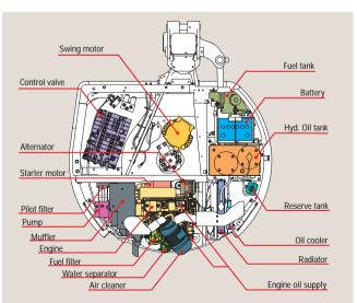
The Zaxis30U-2 and Zaxis35U-2 share the same device layout for easy, efficient inspection and replacement. Inspection points are concentrated for quick daily main-
