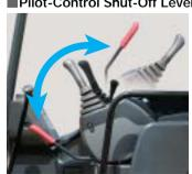
All operations—front, swing, travel and blade—can be shut off by locking the pilot control shutoff valve. This effectively prevents accidental lever control.
